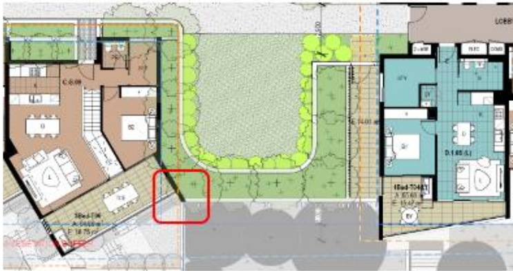
Figure 12 – Minor protrusion of Building C northern-most apartment
